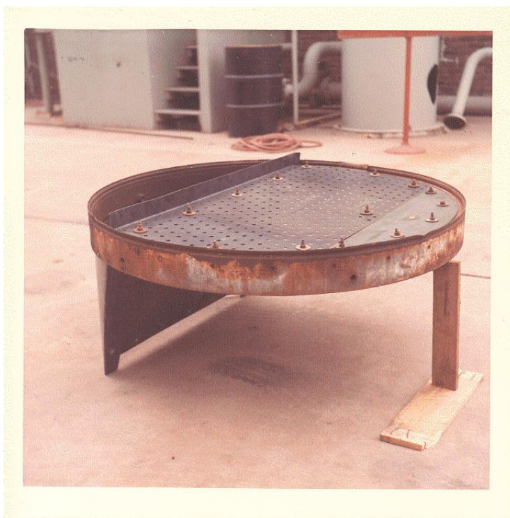
Figure 1. 14% Hole Area Commercial Sieve Tray
