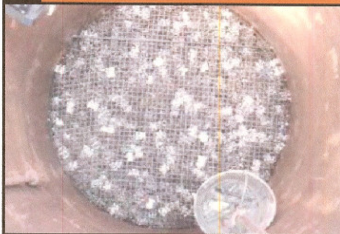
Figure 4. Mesh retainer prevents pieces of random packing from moving around during an upset.
