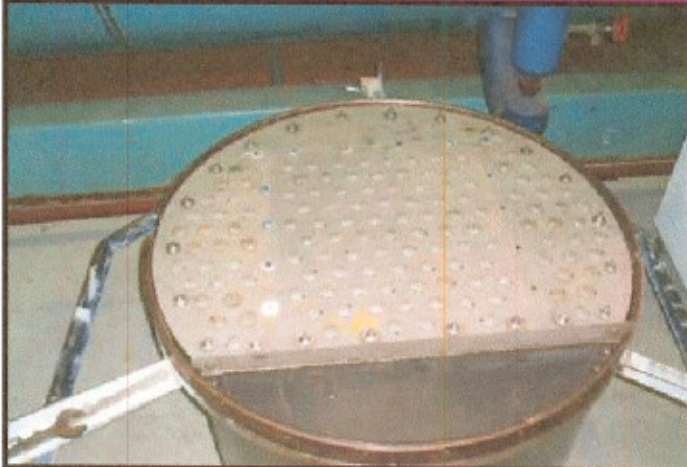
Figure 8. Laying out tray provides a check on fit-up and clarifies its assembly.
