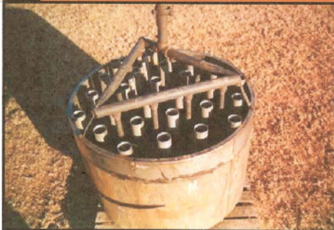
Figure 6. This FRI pan distributor design is commonly used for packing tests.
